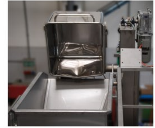
Tray on discharge position inside the receiving hopper of the frying machine
