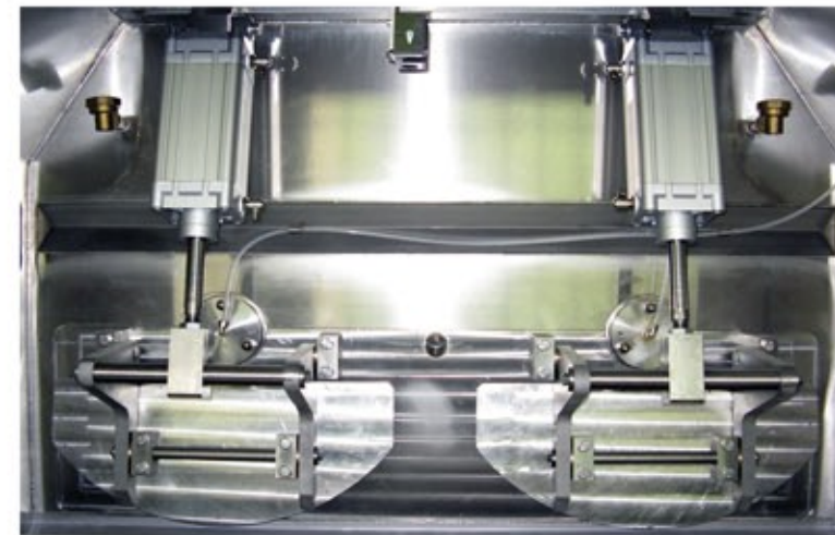
Double discharge hopper (one for each cradle) with pneumatic cylinders powering
