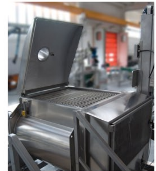
Version of the products' loading directly inside the mixing tank (the safety grid is visible)
