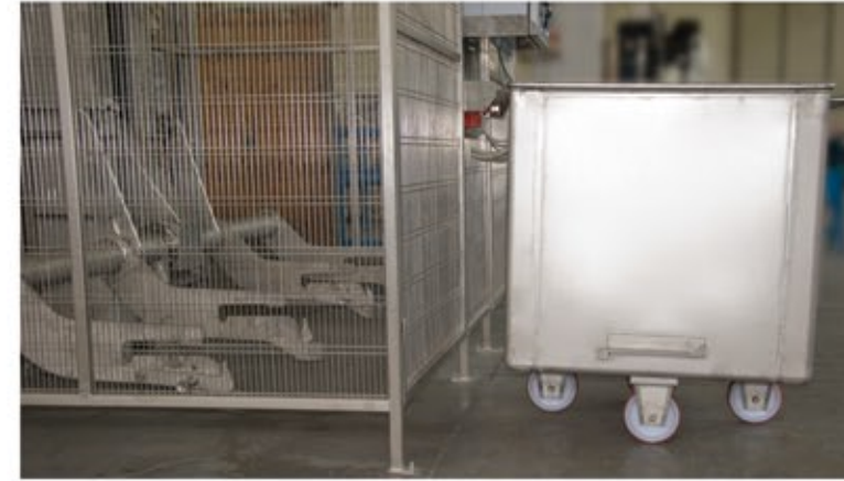
Vegetables' receiving already weighed by means of elevator-tipper for trays
