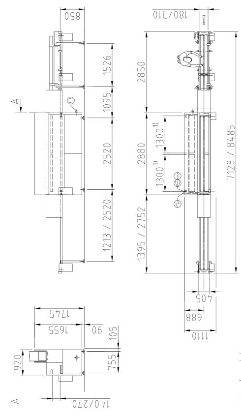
Fig. 2-1, Layout LH (left hand machine)
