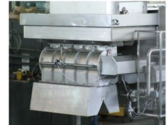
Rotary lock for product discharge
