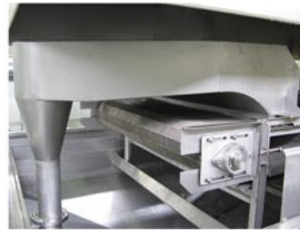
Loading with siphon, fed by hydraulic transport, to keep the product integrity; complete with filtering unit, tank and water return pump.
