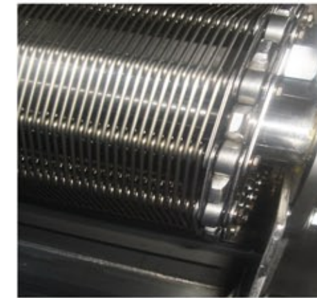
Feeding conveyor with stainless steel belt powered by motorized-gearbox commanded by frequency changer to adjust the product permanence time
