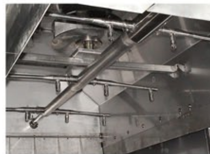
Nozzles for hot water sprinkling on the product for blanching with steam and hot water (only for the model H55W)
