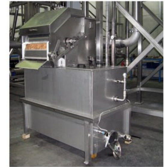
Filtration unit with tank and return pump for the water used by the sprinkling shower system
