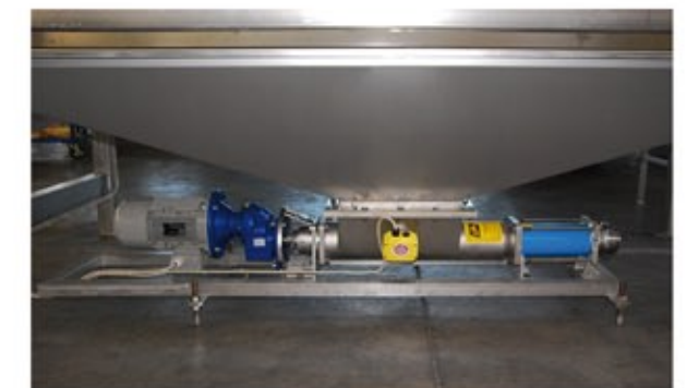
Peeler complete with monoscrew pump for peels' removal (optional)
