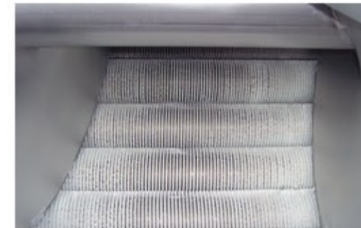
Version of the A81 peeler with rollers covered by brushes (to couple o the Boema steam pressure peeler Mod. SPB)
