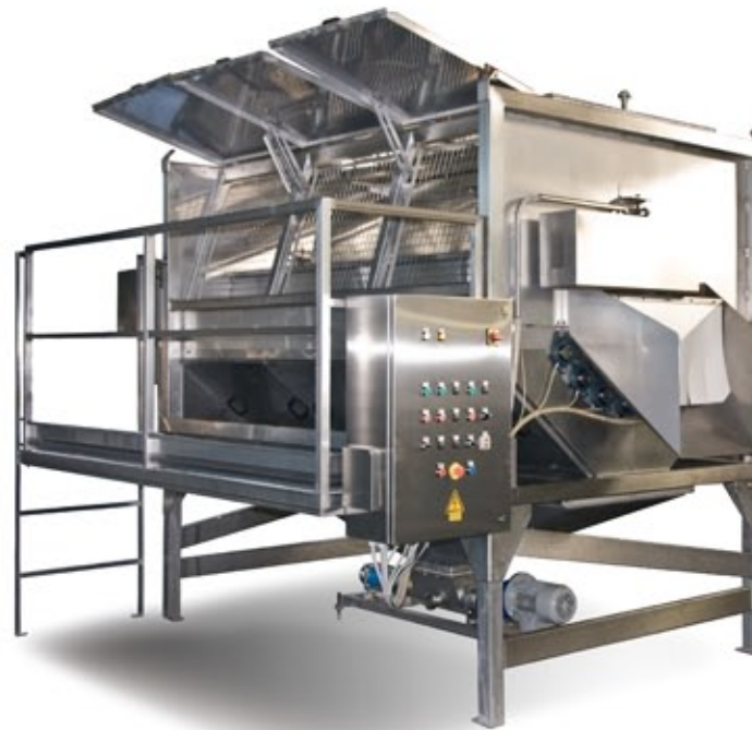
Configuration of the machine opened for inspection and cleaning operations
