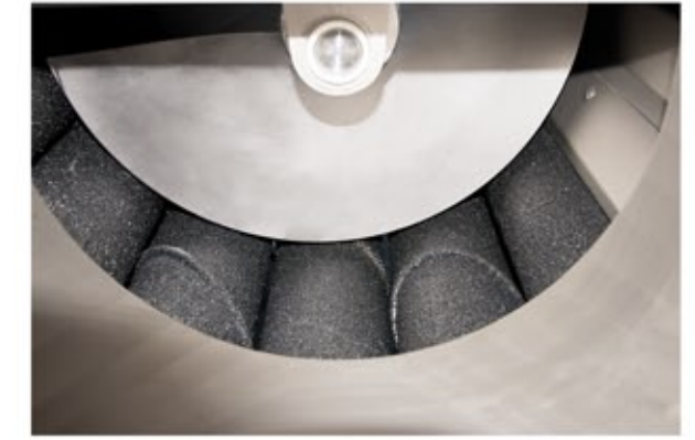
View of the abrasive rollers with the product feeding screw
