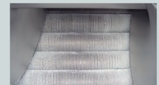
Detail of rollers covered by brushes and installed on the brushing machine Mod. A81
