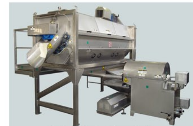
Brushing machine Mod. A81 complete with filtration unit and peels' evacuation pump
