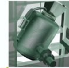
Detail of the peeling pressure container in the loading position
