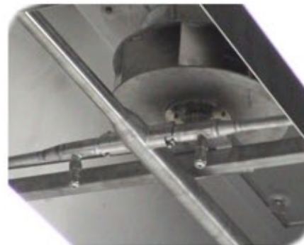
Turbine steam circulation system for product pasteurization (Key Technology patented)
