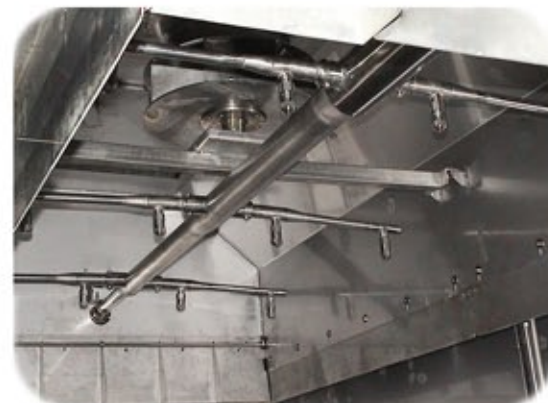
Spraying or "rain" nozzles, according to the kind of product for the rehydration and the further pasteurization.
