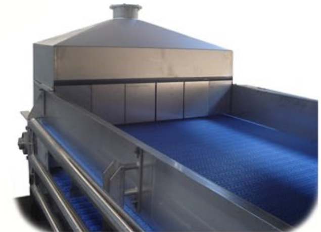
Intralox mesh flat belt at output from the heating section, complete with showers for further sorbate process for product sprinkling (working temperature for "sorbate process" 50÷60°C).
