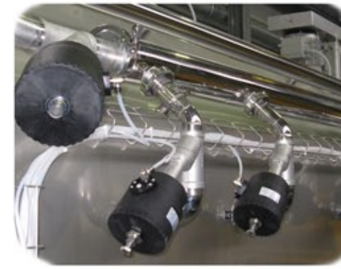
Automatic valves for water distribution by means of nozzles installed on inner manifolds
