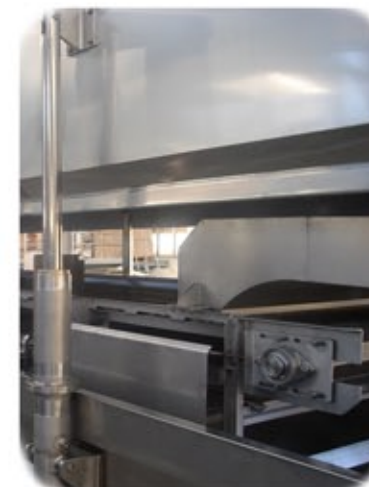
Insulated and sealed (hood) outer envelope, with mechanical lifting system for washing and maintenance operations.
