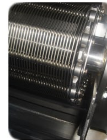
Feeding conveyor with stainless steel belt powered by motorized-gearbox commanded by frequency changer to adjust the product permanence time
