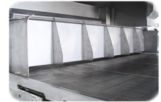
Barriers for the separation of the heating sections
