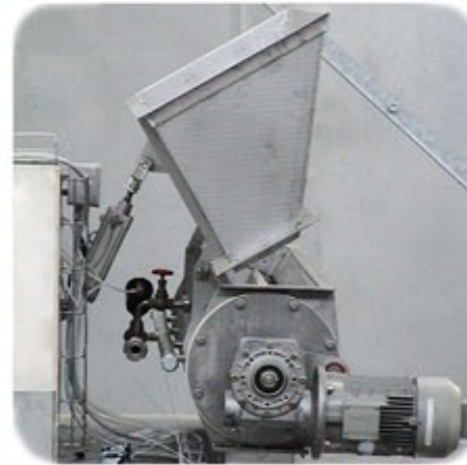
Product loading by means of star valve (optional)
