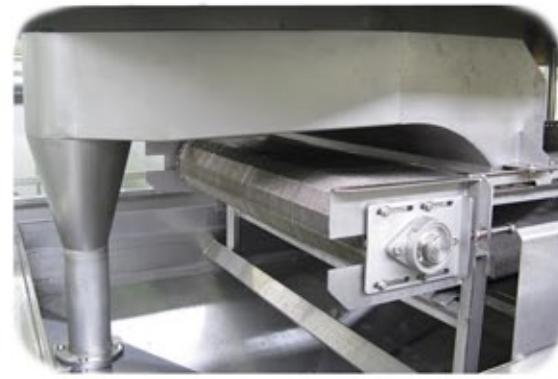
Loading with siphon, fed by hydraulic transport, to keep the product integrity; complete with filtering unit, tank and water return pump.
